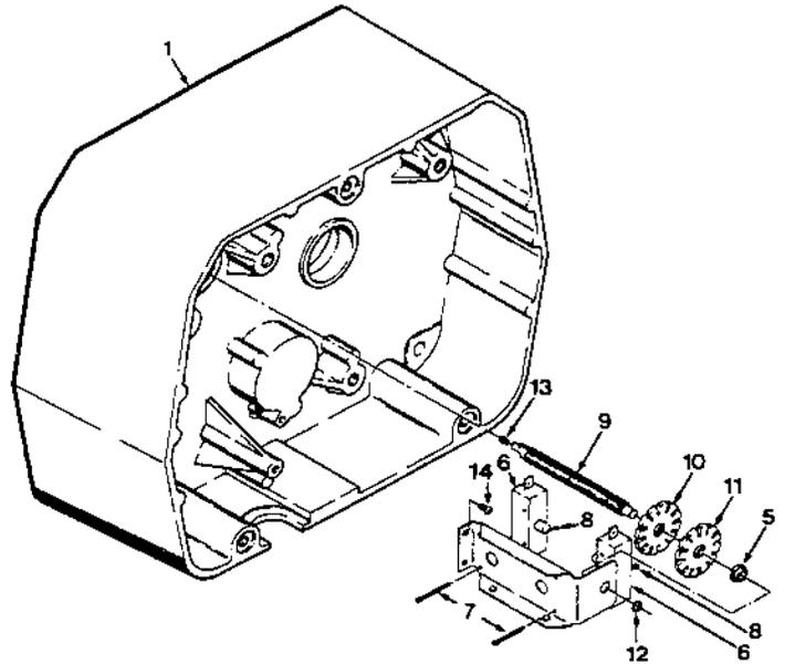
**FIGURE 8-7B. GEARED LIMIT SWITCH PARTS
