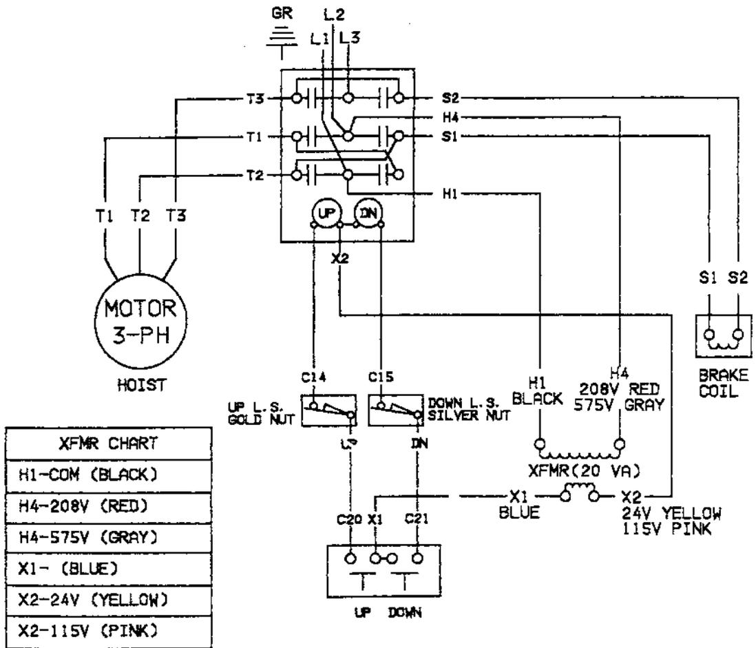
FIGURE 7-2. WIRING DIAGRAM
